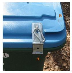
3. Lay the hinge over the lid to mark the best position for the eye of the hasp. Make sure the hinge can be locked and unlocked easily. Pre-drill  $^{3}/_{8}$ " holes in the marked spots on the lid of the can for the hasp eye.
